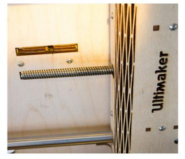
Take the motor out. This part, even with the x4 screws out. With the bed totally down, you can manually rotate the tip of the long screw to take out the motor
