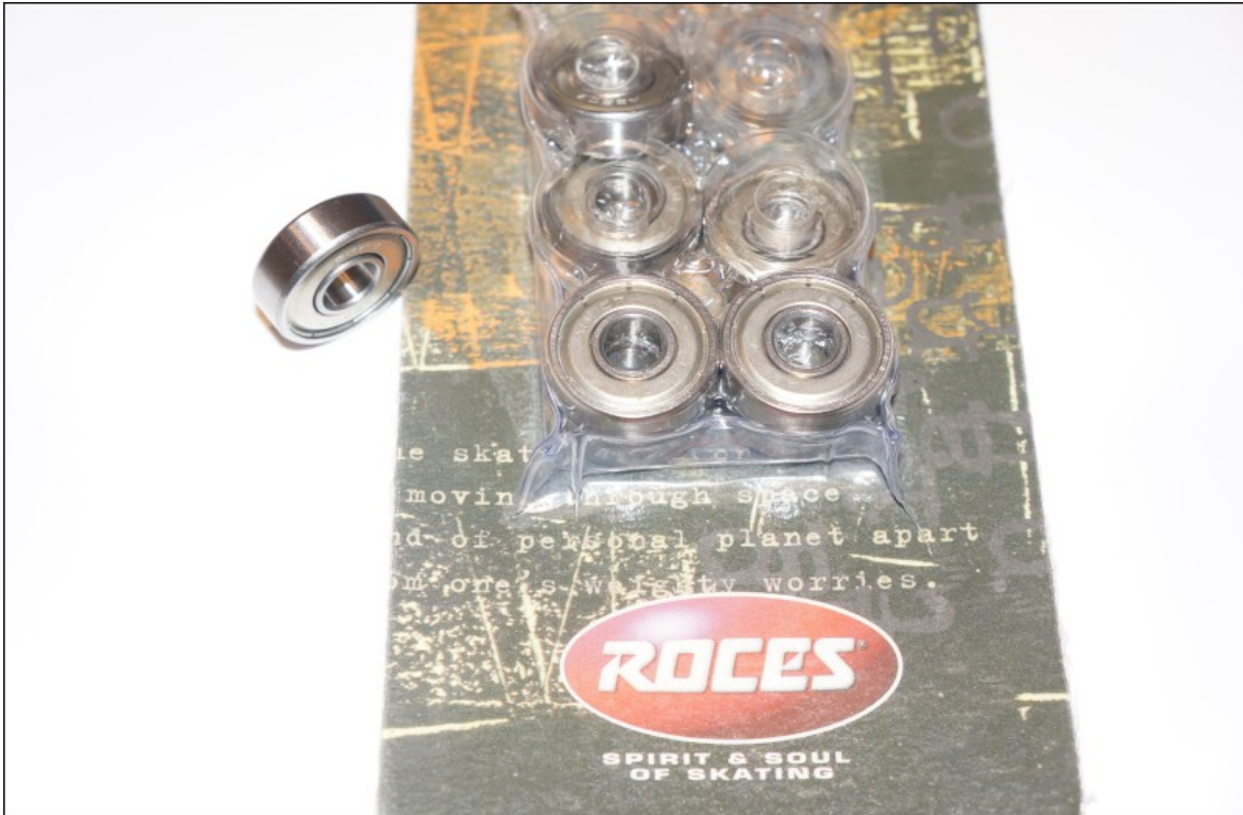
Standard Inline Skater (Skateboard) bearing 22/8 x 7mm width (e.g. ABEC) from local sports store. 4 bearings required
