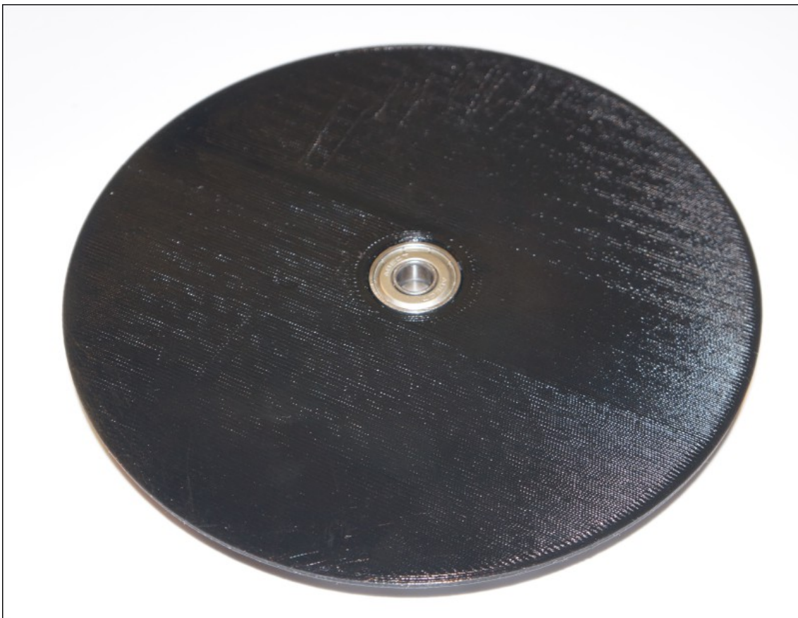
Cleanup the hole in the backside of the disc and press two bearings into the disc carefully Use a third bearing to make sure you moved them completely down into the hole.
