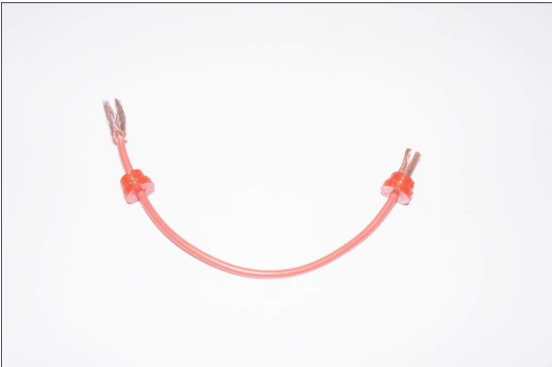
Put in a node and cut it with \sim 1\text{ cm} wire ends
