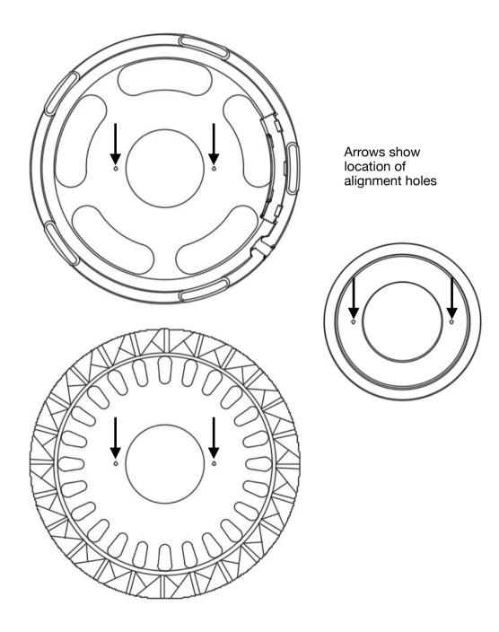
Use two short (~8mm) pieces of filament as **alignment pins** and glue the desired base to the Shade
