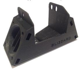
2. Use some (5-7) layers of Kapton tape to prevent the bottom from tue heat of the heaterblock. I additional used a small piece of aluminiumpaper.
