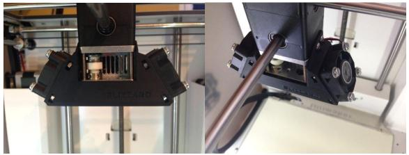
8. Test the correct positioning of the FanMount by heating up the nozzle. Check the bottom of the FanMount. There shouldn't be any deforming. (Here's a picture of mine heated up to 250 °C)
