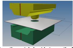
Place the metal sheet between the forming tools, respect the tools marked sides
