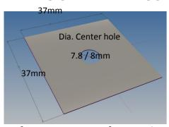
From a beverage can scissor cut a square metal sheet 37x37 mm cutter cut a center hole dia. 7.8 / 8 mm
