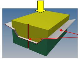
Press down the forming tool By hands or use any clamping tools Mark the outside sheet limit then adjust By cutting with the scissor adjust With a cutter if necessary **Carefull your fingers, the metal sheet**
