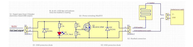
R2 & R3: Voltage divider to convert the 19V signal to ~10V for the MosFET
