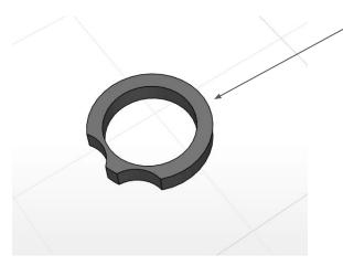
this washer can be placed in here if the arm is loose. you can make it as thick as required to eliminate the play.
