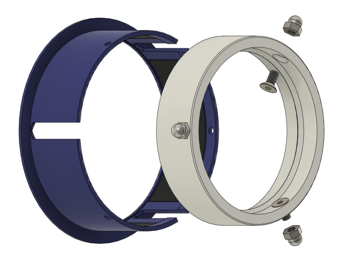
Insert the M4 domed nuts into the hexagonal stencils of FRONTELEMENT, guide the 8mm M4 screws through the holes on the other side and screw them tight (don't overtighten!). Now push FRONTELEMENT with the threads first into the rear of FOCUSTUBE, the domed nuts guiding through the longholes.
