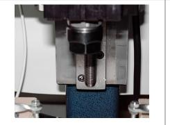
1. Remove bit from spindle.
