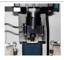
2. Push camera on to spindle and connect camera to USB port of computer.
