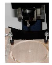
9. Remove the camera from the spindle and put the bit into the collet and home the Z axis.
