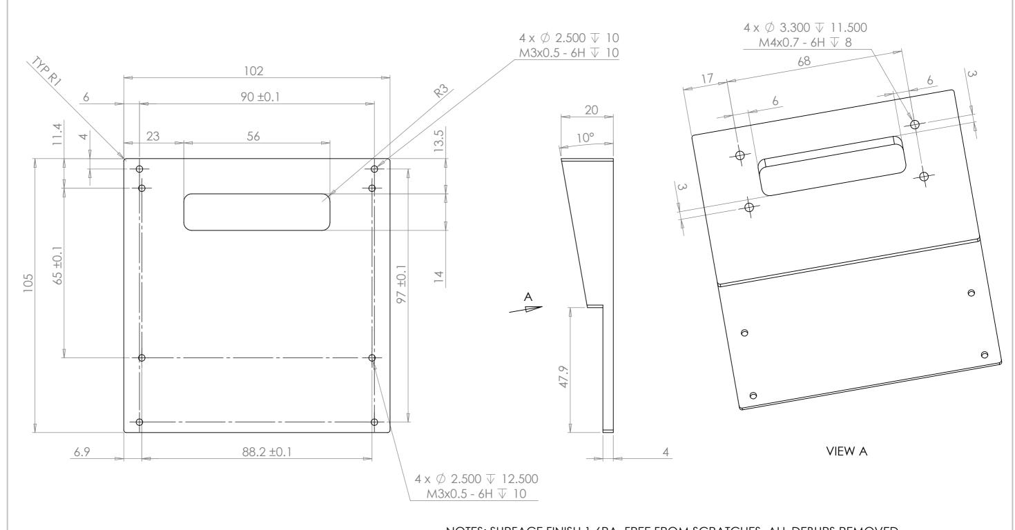
NOTES: SURFACE FINISH 1.6RA, FREE FROM SCRATCHES, ALL DEBURS REMOVED BEAD BLAST AND CLEAR ANODISE.
