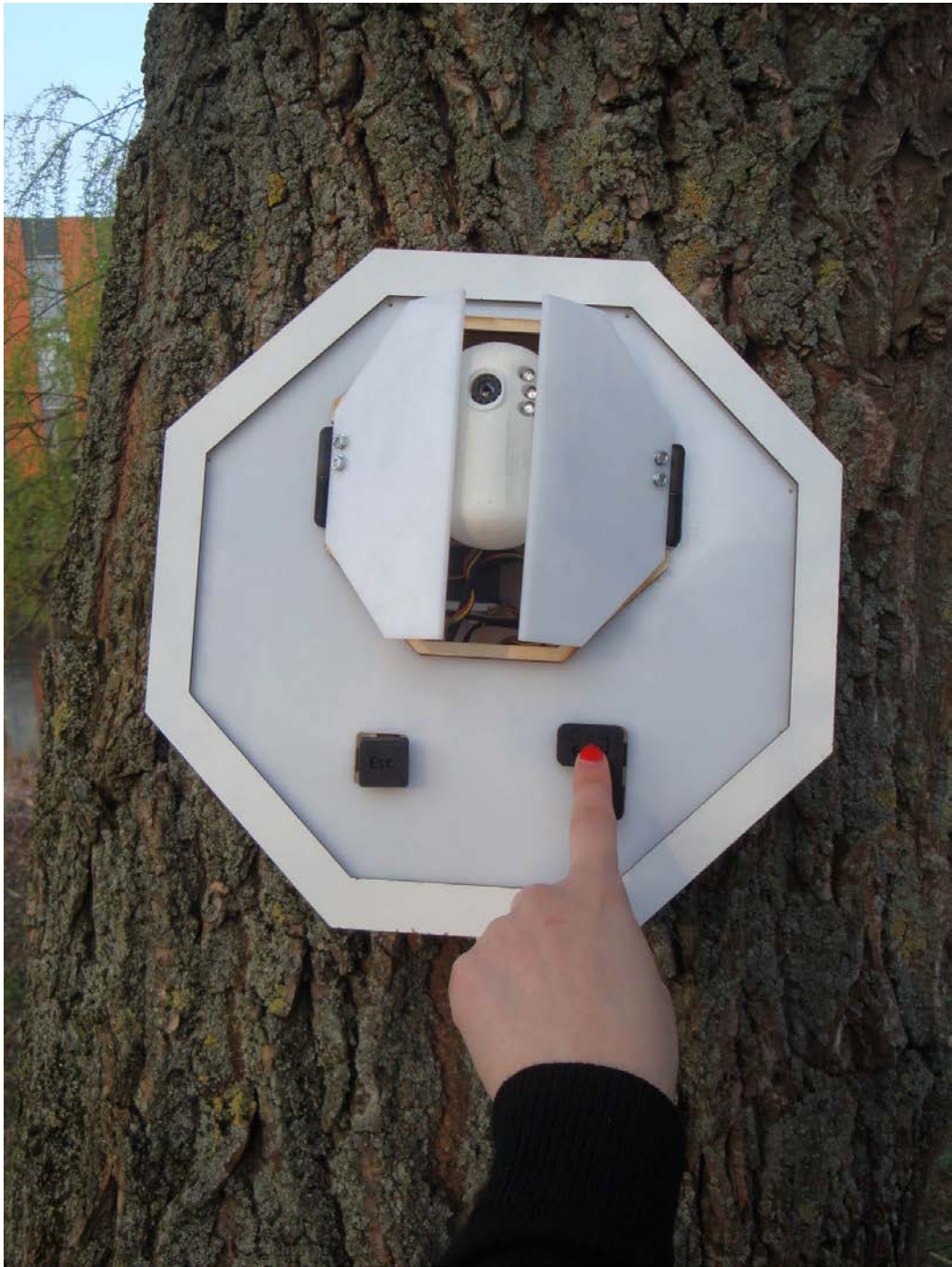
Figure 61: completed first version of the sign on/off device, FabLab user pushes ENTER-button
