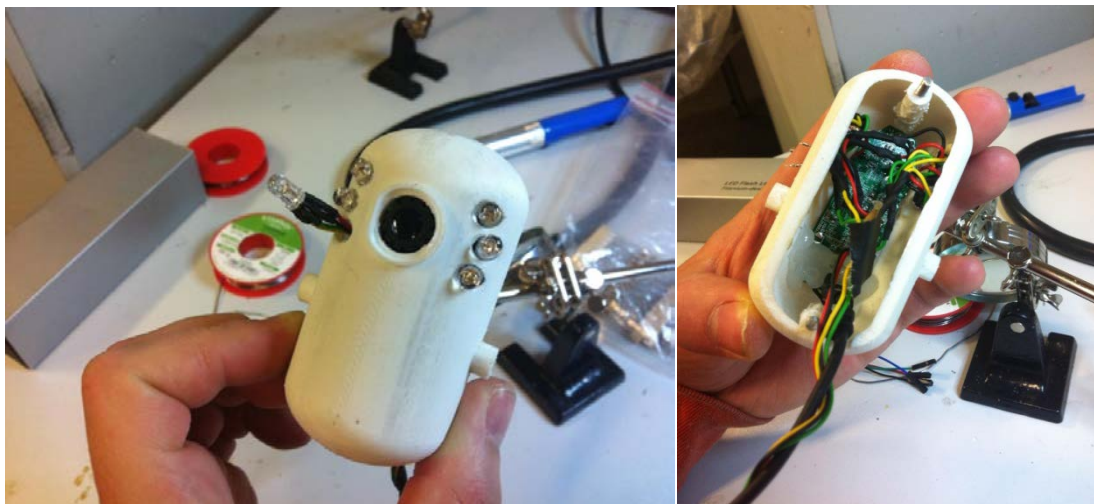
Figure 53: realization of the case for the webcam and the RGB LEDs
