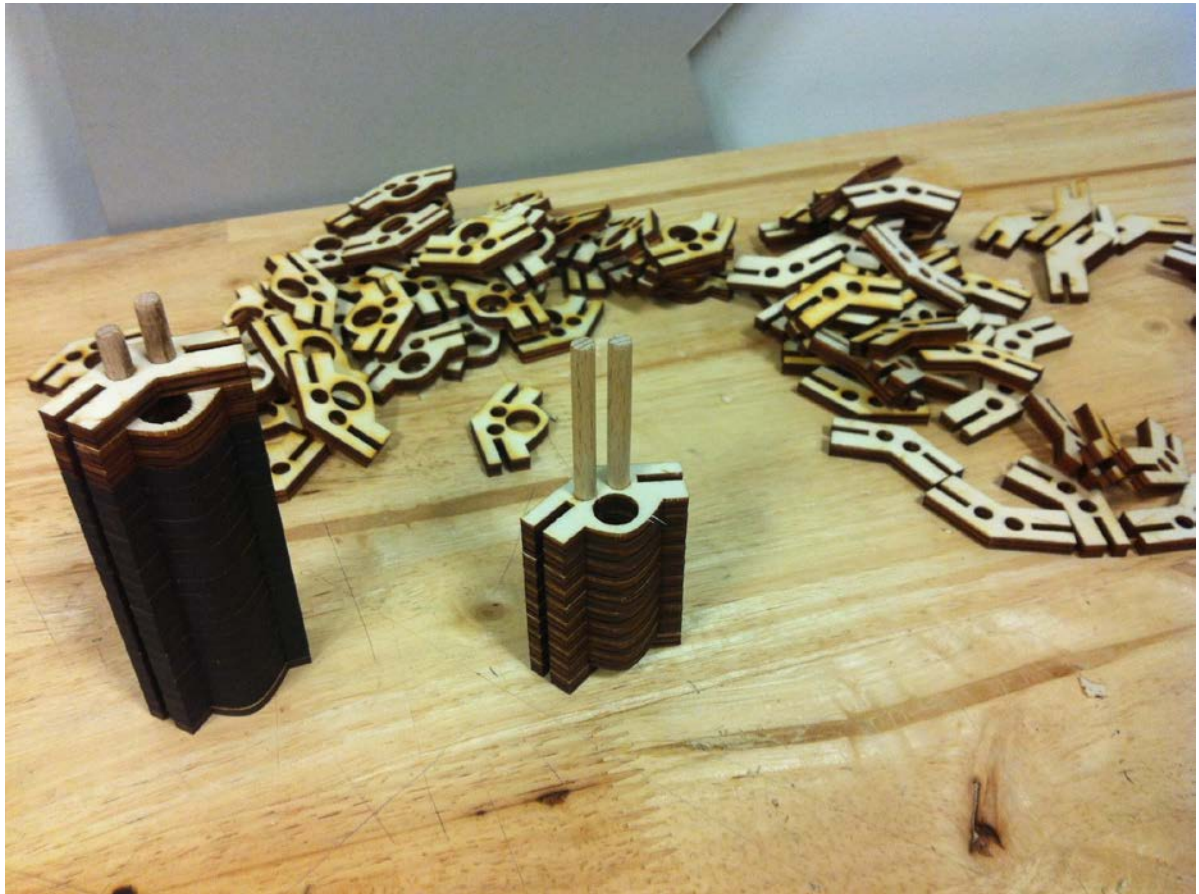
Figure 45: realization of the corners connecting the walls of the case
