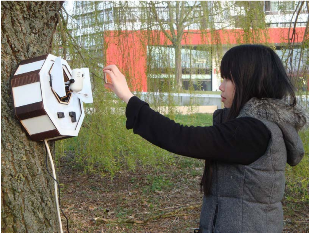
Figure 62: completed first version of the sign on/off device, FabLab user holds member ID with QR code in front of the webcam
