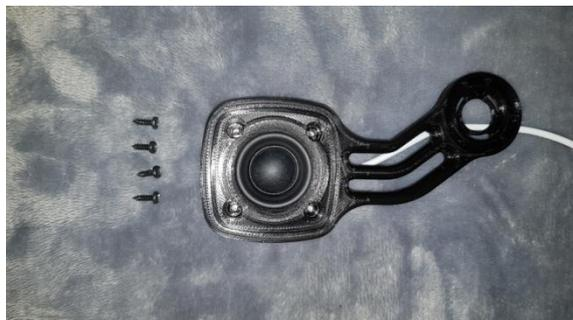
Insert the speaker frame (GT\_Air\_Speaker) into the socket of the speaker arm.
