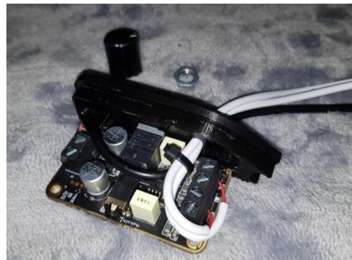
Fasten the amplifier with the screw nut.
