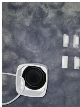
Insert the mounting ring (GT\_Air\_Cover\_Reflex) into the cylindrical cutout of the cover.
