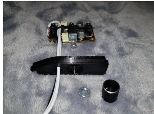
Connect the right 50 cm audio cable to the left upper socket of the Droking PAM8406 amplifier.
