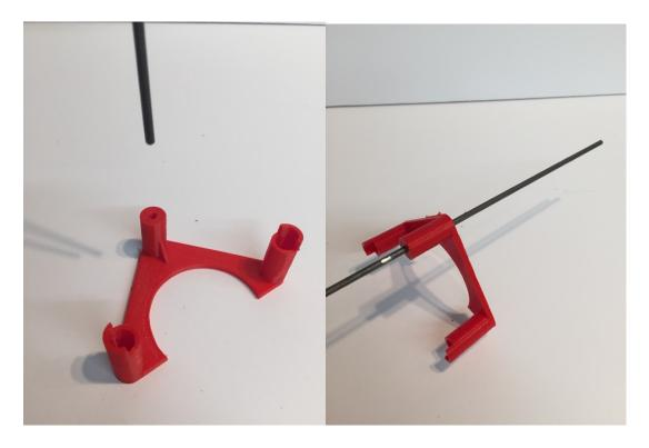
GRAB A ROD AND SLIDE THROUGH STAND. ANY ROD WILL WORK AS LONG AS IT'S STRAIGHT AND WON'T BEND EASILY.
