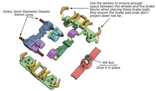
**Step 2**Slide the wheels onto the Ø4mm 54mm long dowels, and allow sufficient to stick out where it can engage with the recesses on the side panels. This is typically 4.5mm each side
