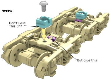
With your two bogies in hand, add the two bogie wire terminals. These are where your wires will connect. The two bogie hubs can be installed. These are not glued. Leave a little looseness in the screws so the bogie pivot will turn. It is probably worth adding a washer in between the bogie and the bogie hub to allow smooth rotation.
