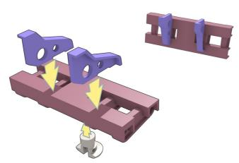
Assemble the two buffers. Use the deck assembly to ensure the spacing between the webs is correct.
