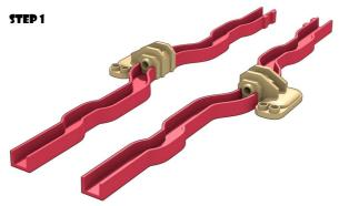
On a good flat surface glue the side rails onto the Undermass Left and Right components. Just be aware which way the wobbles go and where the two lugs on the back of the "UnderbarsBack" components are. It will pay to use a straight edge along what will be the top surface of the "Underbars" to ensure the deck is glued straight.
