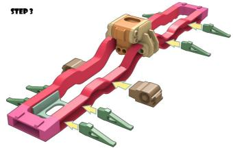
Add the footplate supports and the two battery tray terminal blocks. To make things easy, lay the assembly on its back as shown and pack up the footplate supports with some cardboard so they are sitting flat.
