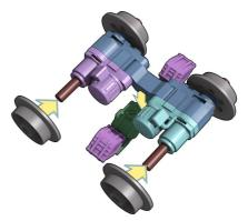
**Step 3**Drop the upper cross piece down onto the leaf springs and slide the side pieces into place.
