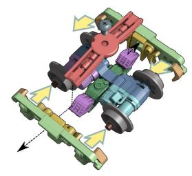
**Step 4**Well, actually there is no step 4. This is just to illustrate how the assembled bogie should look.
