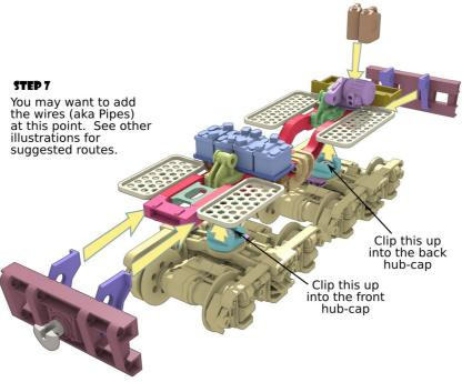
With the bogies installed and the assembly sitting on rails or at least something that will allow it to sit as it would on rails, glue the buffers in place allowing space below them so they're not dragging on the ground. Don't slide them too close to the bogies either, you still want the bogies to be able to swivel a bit. Add the wires to simulate the cable routes. Below are the routes I used on mine.
