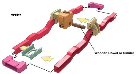
Use the small Ø4mm dowel stub to help locate the two side sections. Glue the endcaps and FrontWeb in place.
