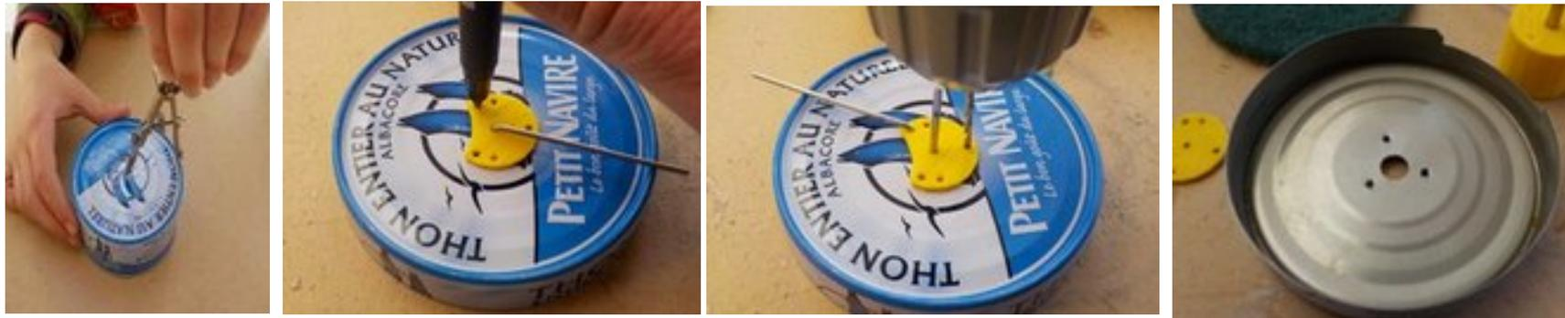
The box superior can be cut with a pair of shears with sheet steel or certain chisel, with defect cut in the saw has metals and to fold the sheet steel Here the guide of the "piston deplaceur" is made in ugly of an axis of 3mm and of a tube diameter 3mm (Rep 7)
