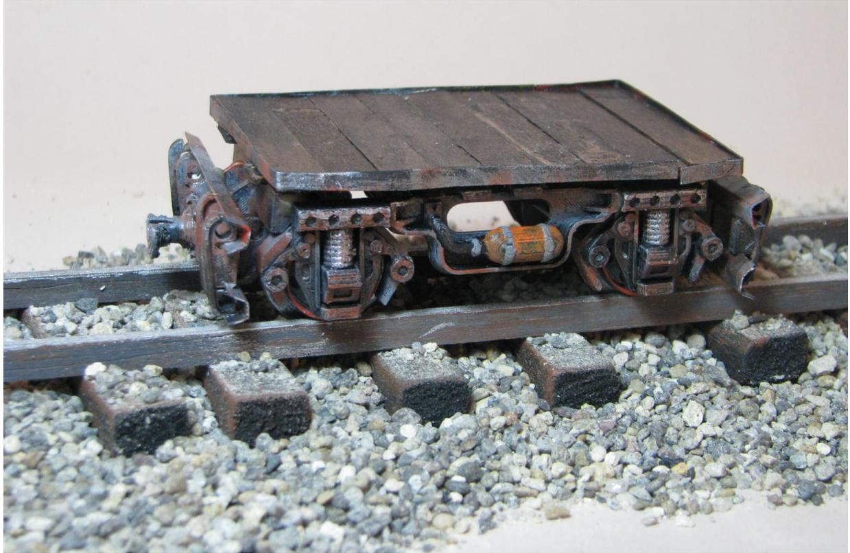
Encouraged by the success of the Mine Trolley Prop for stop motion project, I decided to design some wagons to fit the Mine Trolley. The 3D printed model presented here is a chassis that can be fitted with any other sort of top. For this first version, I just made a simple flat-deck using ice-block sticks.
