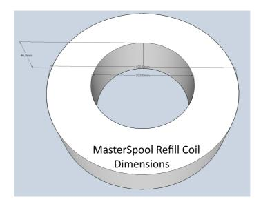
Suggested dimensions for the refill coil to use the MasterSpool holding system.
