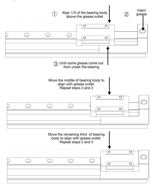
• Slide bearing back and forth to spread the grease evenly. Repeat above as necessary.
