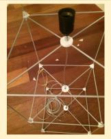
Attach the powercord to the fitting and pull it through the center\_pieces
