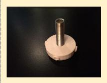
Take one of the middle\_pieces and a piece of screw-thread that is made for a fitting and screw it in gently.
