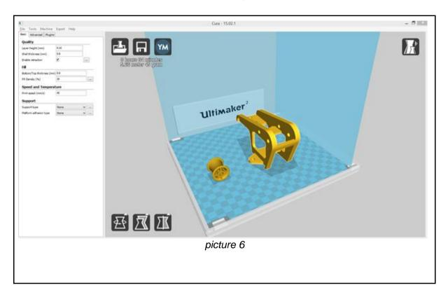
Click on the pulley and use the Rotate button to rotate it 90 degrees. (see picture 7) Click on the bracket to rotate it 180 degrees. The rotation is necessary for the print. If you don't rotate the bracket, the print takes very long because you have to print a bigger support structure.
