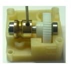
Note: the bearing F has to align with the grip wheel shaft on the right. This will require forcing the gear wheel and spacer down on the grip wheel shaft.
