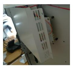
After unscrewing the 2 bolts you can remove the bottom cover.
