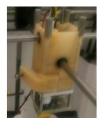
Try to move the flexible axis again to make sure the movement of the worm wheel and the hobbed wheel assembly is withouth obstruction.
