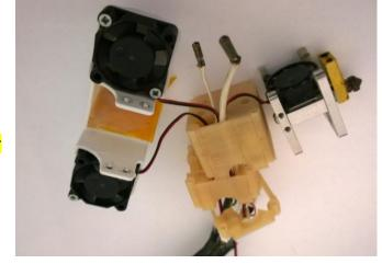
fan connectors. Take the heater and temperature sensor and guide them through the printed head as well.
