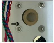
Take the rings T and insert bolts O into them. Slide them into the holes of the original feeder motor from inside the chassis facing outside. Slide the motor Spacer P-G over the bolts sticking out, then the Motor Bracket K and finish with the bolts O. secure the connection but do not overtighten.
