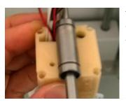
Take the complete head and separate printed parts P-A and P-B from P-C (while keeping P-A and P-B together!) and press it below the Y axis bearing. Make sure the cables are all on the lef of the bearing. Take printed piece P-C and slide it down the cables so it connects on top of P-A and P-B. snap it together so it is a tight fit. Depending on the amount of cleaning up you have done this will stay together or you might have to hold it.
