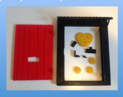
Step 2: Drill (3mm) hinges on door and mailbox parts. Make sure they can move freely on 3 mm wire.
