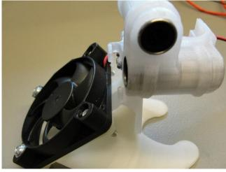
Now, guide the wires of both fans through the wire guides, and through the tunnel and towards the center of the mount:
