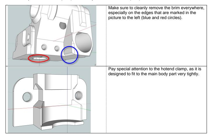
After that, make sure your hotend fits into the mount. If you attach the clamping bracket to fix the hotend in place, it should fit either just fine, or leaving a very small gap (0.5mm max). If there's a gap, make sure all the surfaces making contact with the hotend are very clean. You can close a very small gap when tightening the screws, but make sure you don't need too much force or you will damage the threads.
