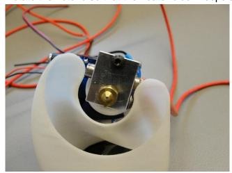
Now you can tighten the screws holding the hotend clamp.
