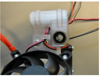
After that, tighten the two screws to fix the fanduct mount and secure the wires in their guides.
