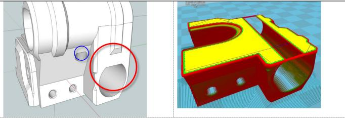
Bridging-helpers for the main linear-bearing tunnels (red circle). These supports help a lot with the bridging part, but need to be removed in order to get the bearings in. Remove all four supports (two on each tunnel).
