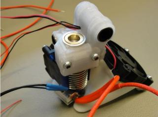
Rotate the hotend so that the heater block keeps a good clearance to the cooling fanduct:
