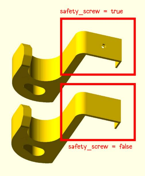
If you choosed the hook with rectangular "bracket", it may be good to have a safety screw to lock hook into place. If you need it, type "safety\_screw=true" in "extra settings". It will use the screw parameters defined in "screw-holes" part.
