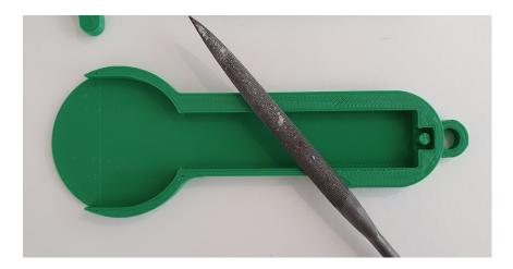
Step 4 – Remove the dust from the filing and then put a small blob of silicone grease here (see picture below). If you don't have any skip this step.
