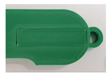
Step 12 - Clean up any sharp edges with a file. On some printers the text can remain quite sharp (check the "-" in particular).
