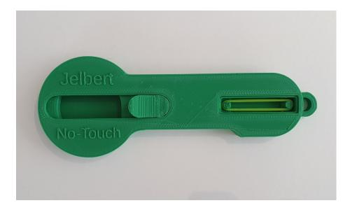
Step 9 – File the elastic band "door" edges until it fits into its slot...
