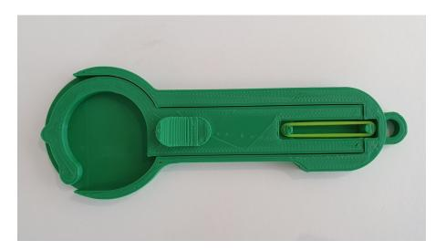
Step 7 – Put a bead of super glue around the edge of the base assembly...
