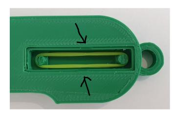
Step 11 – Slot the elastic band door into place and hold firm for a few seconds...
