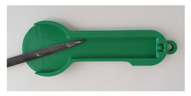
Step 3 – Use the flat file to make the top surface of the base smooth ready for gluing...
