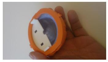
Insert one of the Partition clips. The round edge should sit nicely between the front ball and the crystal, holding the crystal firmly in place.
