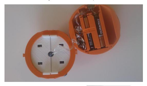
Match the clips up to the flat edge of the battery pack clipping in place one side before the other. This will require a little force to bend the clips a little but don't overdo it or you will break them.
