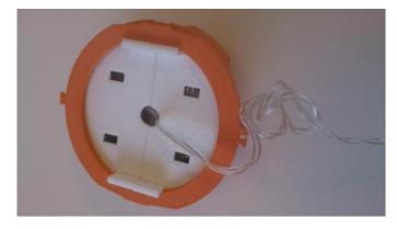
Slot the switch and battery connectors in to place in the battery pack and battery door. This should be done before inserting the batteries but the photos below are from an already made Matrix.
