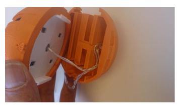
Put the excess wire into the cavity in the battery pack, there is a small groove for the wire feeding from the front ball
